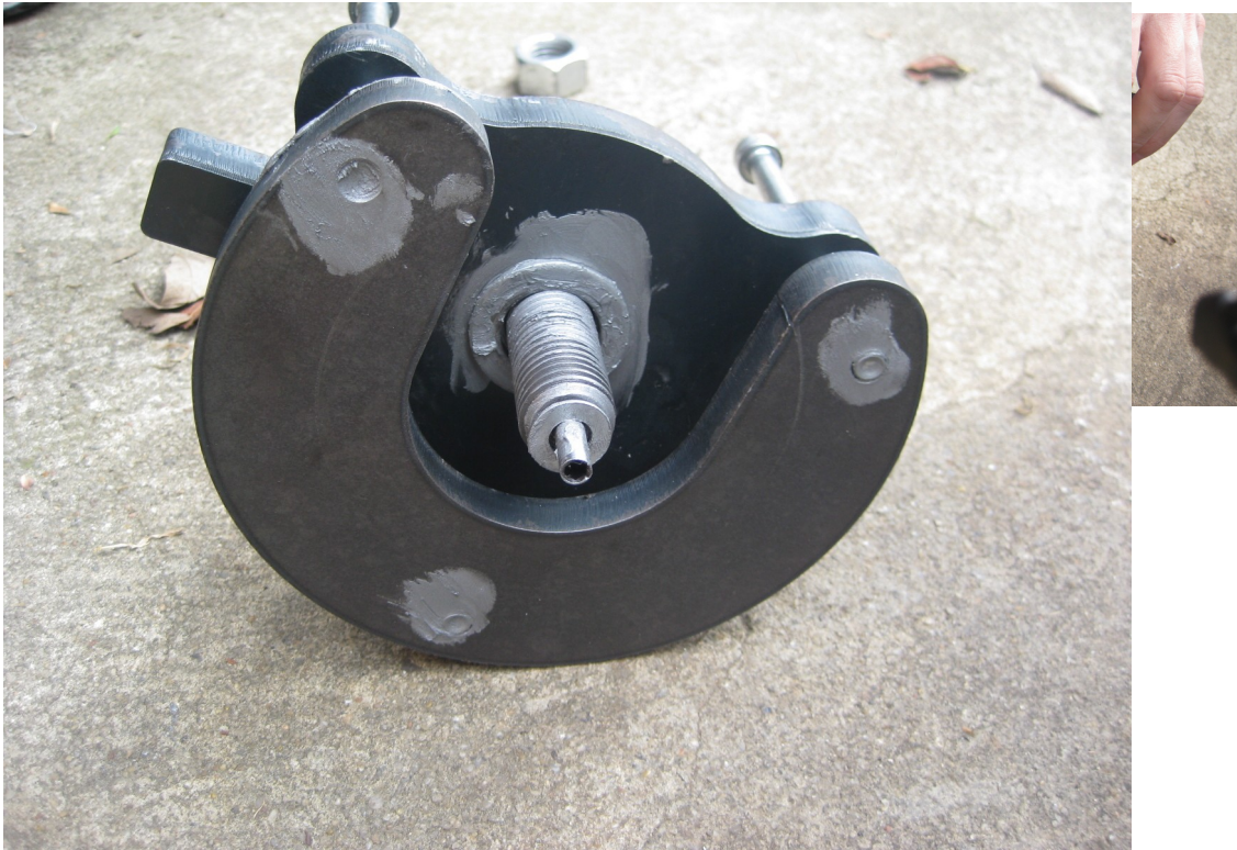
Step 6 – Removing the pulley
