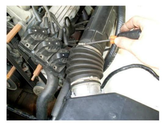
**Step 2** - The lid of the airbox has 5 clips that hold it to the base of the airbox. Flick down these clips and remove the lid of the airbox.
