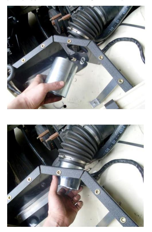
Step 8- Insert the pod adapter pipe into convoluted hose and tighten hose clamp.
