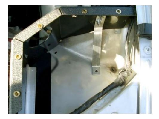
**Step 2** - Drop the new performance enclosure into position as shown. Make sure the 3 mounting holes are aligned. 2 of them are in the plastic base of the enclosure, the other is in the bracket.
