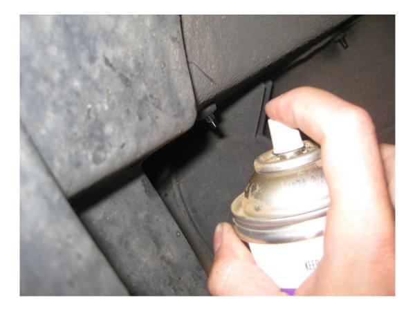
Using a steel wire brush, clean the bottom of the studs such that the threads are relatively clean. Then spray the studs again using chain lube or any other industrial type lubricant.
