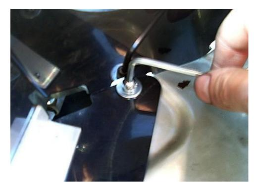
**Step 4** - The support bracket for the enclosure was inserted in the following way. Place the 2 screws through the wall of the enclosure.
