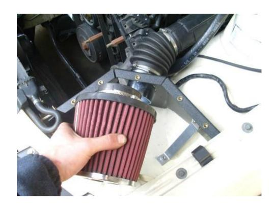
**Step 9** - Slide pod filter over the adapter pipe and tighten with hose clamp.
