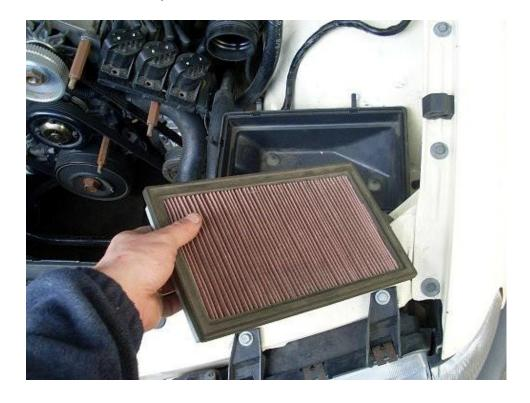
Step 3 - Lift out the air filter element by hand.
