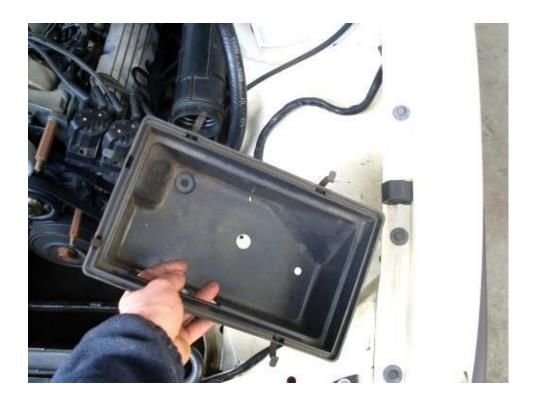
**Step 5** - After removing the base of the airbox, 3 rubber bushes with protruding studs will remain. DO NOT attempt to remove these until they are cleaned properly from underneath the guard as this may damage the stud.
