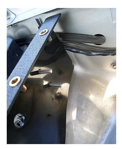
Place a flat washer, spring washer then the nut in that order. Tighten the nut while holding the head of the screws using a flathead screwdriver.
