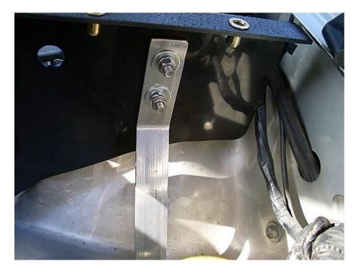
Place the flat washer, then spring washer onto the base of the enclosure over each hole, then insert the cap screws provided with the support bracket through the base of the enclosure and tighten with allen key.
