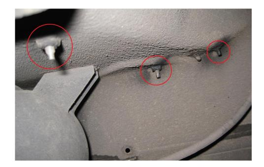
Firstly locate the studs beneath the guard as shown in the image below.
