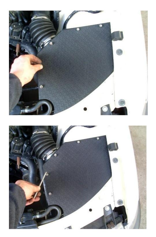
Insert the button head cap screws and tighten using allen key.
