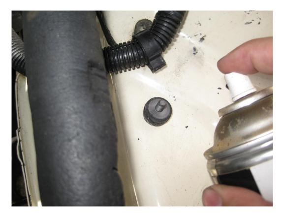
Using pliers (or vice-grips if required) grip the rubber bush, DO NOT grip the actual stud as the stud assembly is made of up two pieces which may shear. Turn the studs anti-clockwise to remove them.
