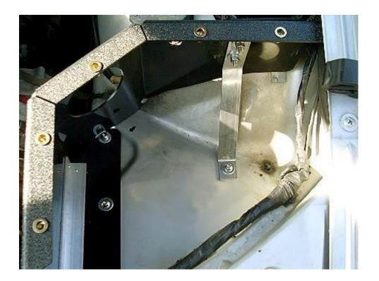
**Step 5** - The plastic inlet pipe is supported by a bracket that is bolted into the side of the engine bay. The pipe must be lowered for proper fitment of the new enclosure. Bend this bracket down to allow the pipe to drop by about 20mm at the end that will meet the airbox.
