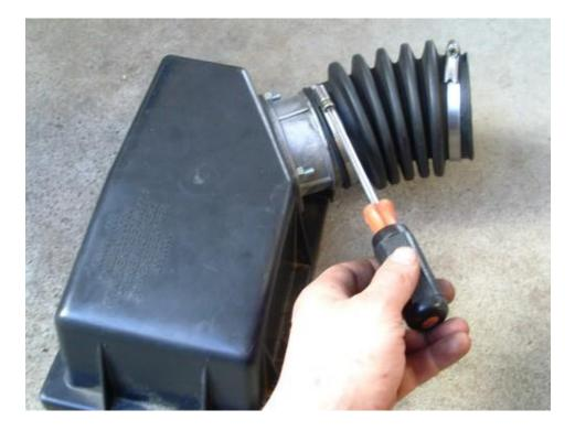
**Step 7** - Fit the convoluted hose to the end of the intake pipe. Tighten the hose clamp with a screwdriver.
