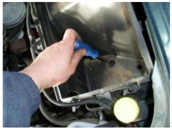
**Step 11** – Pull out the wiring loom that is held in 2 places on the box by clips.
