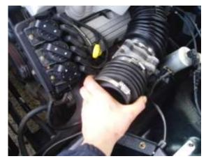
**Step 5** - Insert pipe piece into rubber adapter & tighten hose clamp.
