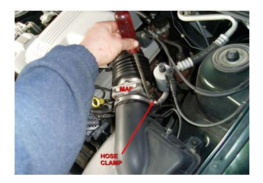
**Step 5** - Remove the hose clamp completely & pull the top cover out away from the MAF as shown below.
