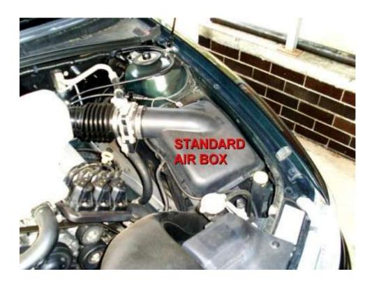
**Step 1** – disconnect air temperature sensor from the top cover.
