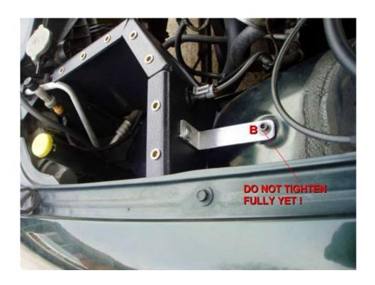
NOTE: Please rotate the MAF anticlockwise about 90 degrees as shown in the image below for adequate clearance. Also notch the rubber intake hose such that the new notch sits on the tab of the MAF which has now been displaced.
