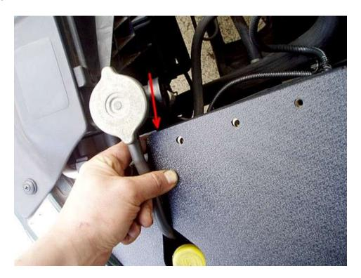
**Step 12** - With all lid screws in place hold the box in a position so that the yellow filler cap is approximately in the middle of the hole of the lid & finish by fully tightening the bracket mount at the back with an alley key (simultaneously either using you other hand or having someone assist you).
