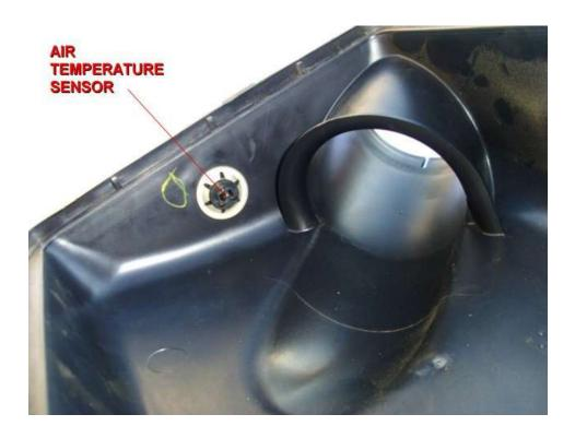
**Step 2** - Lift off each strip of the retainer clip holding the air temperature sensor using a screwdriver.
