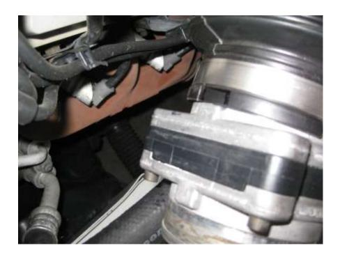
**Step 4** - Insert rubber adaptor onto the MAF and tighten the hose clamp. Carefully tighten over the adaptor tube such that it doesn't leak between the tube and the hose.
