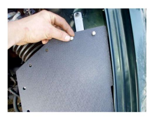
**Step 9** - Squeeze the box with you hands to make the holes of the lid aligned with those of the box. The box is inherently elastic & designed to flex into place.
