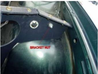
**Step 3** - The bracket bolts into the car body at position B via the original mount by a socket headed cap screw using an allen key. Insert the cap screw BY HAND all the way down but DO NOT FULLY TIGHTEN YET by allen key. LEAVE IT LOOSE. The mount at position B allows for some movement & will need to be adjusted for optimal placement at the end of the installation when everything else is in place.
