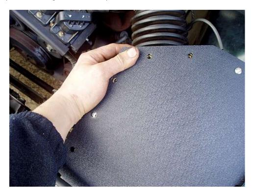
**Step 10** - For the final holes at the front, place your finger under the lid & bend the side wall of the box to align the holes.
