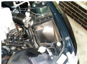
**Step 7** – Lift up the standard air intake by popping out the 2 clips at the front & remove it.
