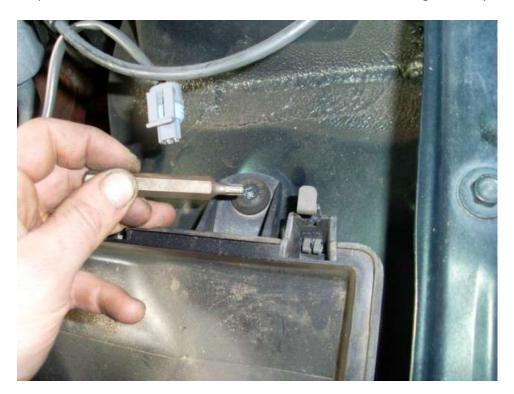
There are 2 torx fasteners to be removed. One is up at the back & the other is inside the base at the bottom as shown below
