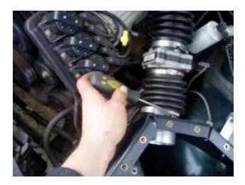
**Step 6** - Place pod filter onto the pipe piece & tighten the hose clamp.
