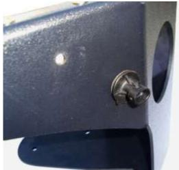
**Step 5** - Place the retainer clip back on the temperature sensor & firmly squeeze them together through the wall of the enclosure.
