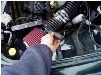
**Step 7** - Place the lid of the box approximately in the correct position & check that the radiator overflow hose will reach its fitting beneath the radiator cap.
