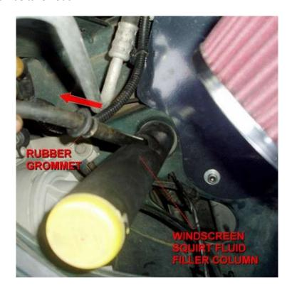
Position of rubber grommet controls how much of the hose will stick out of the filler column. To slide the grommet along the hose, the hose must be pulled & stretched to thin it out.
