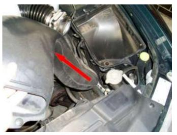
Step 8- The next step is to remove the base of the air box from the mounts using a torx tip
