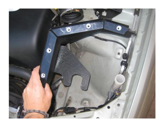
The CAI enclosure naturally sits in a position such that the slot in its base easily fits around the groove in the vehicles bodywork.
