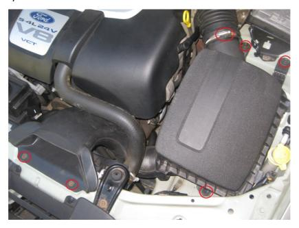
Start by loosening the hose clamp on the hose which connects to the lid of the air box.
