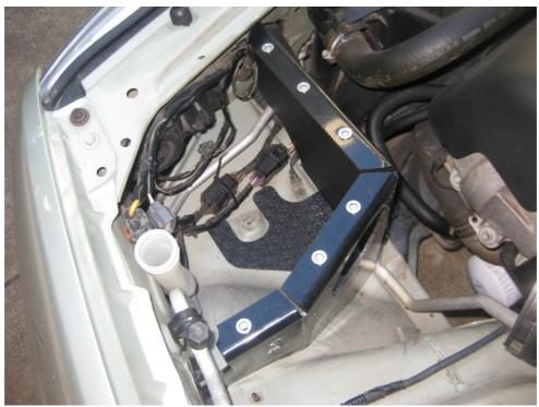
The side of the enclosure facing the engine should sit flush with the chassis rail as shown below.
