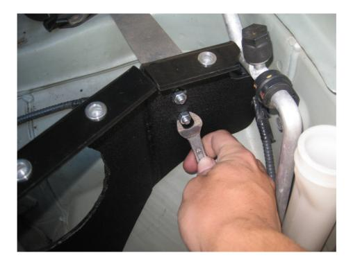
Use the nuts to mount the bracket onto the enclosure and secure using a spanner or socket wrench. Secure the top of the bracket using one of the cap screws provided.
