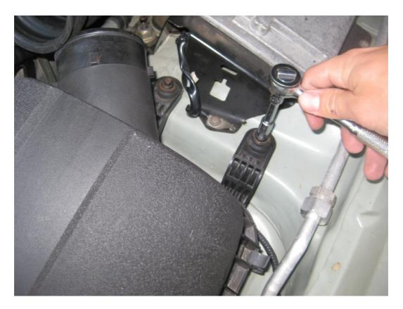
Note the bottom bolt behind the headlight as it may not be clearly visible (below right).
