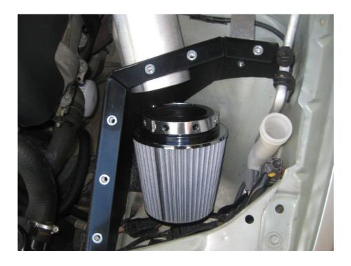
Tighten the hose clamp supplied with the filter..
