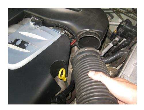
In order to maximize air flow, the largest possible size pipe has been supplied but may be a tight fit. The use of a flat head screwdriver while pressing it up against a surface will make insertion easier. Lining the outer edge of the tube with a lubricant such as oil or Vaseline will also help insert the tube. If insertion is difficult, leaving the end of the tube in a bucket of hot water will let the rubber expand enough to insert the tube.
