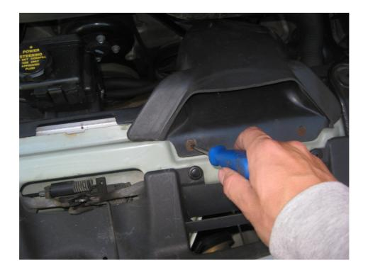
The intake snorkel can be removed by twisting and rotating it such that the joint at the bottom of the box dislocates as shown in the images below.
