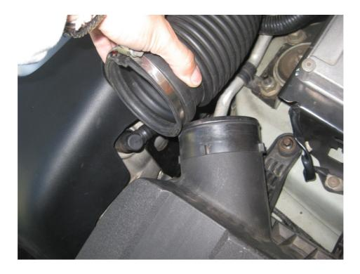
Proceed be removing the two screws on the intake snorkel as shown below
