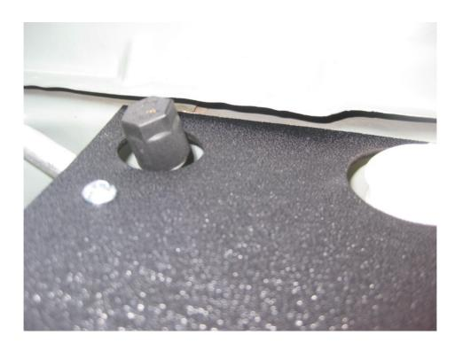
Place the top right-hand corner of the lid under the quarter-guard flange first before placing it over air-con receiver cap and washer bottle respectively.
