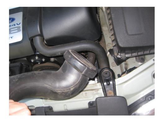
At this stage only the three bolts holding the box itself are left to be removed by use of a socket wrench.
