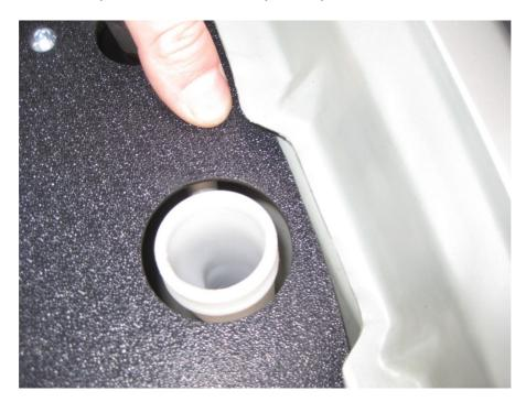
Insert the screws into the holes and first finger-tighten all screws while adjusting the enclosure accordingly such that all holes align.
