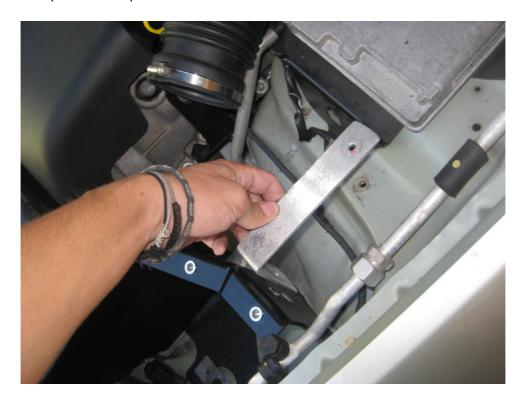
2 small screws and nuts are provided to mount the bracket onto the face on the enclosure.
