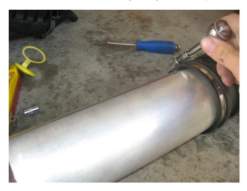
Fit the intake through the CAI enclosure before attaching it to the plastic intake manifold as shown below.
