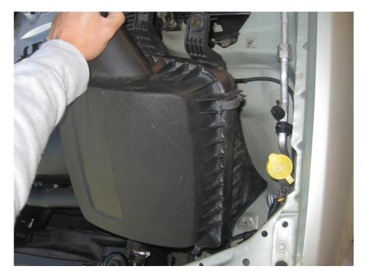
Once all 3 bolts are removed, the air box can simply be lifted out as shown below.
