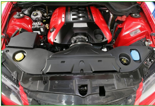
OTR installed on E2 GTS with VCM Infill Panel and Fascia Panel Kit.
