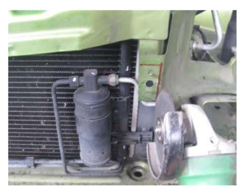
The material removed includes one of the bolt holes for the headlights. The headlight will still be supported by 2 other bolts making it still very rigid. An extra support may be made up.
