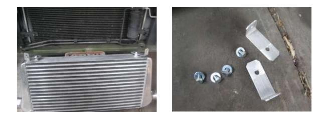
Using self tapping screws, drill the screws into place as shown below making sure the core sits evenly between the headlights.
