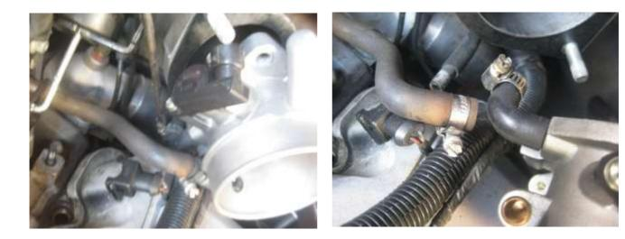
The throttle body can now be removed from the elbow. It will still be attached by the throttle cables but will enable itself be be maneuvered out of way.
