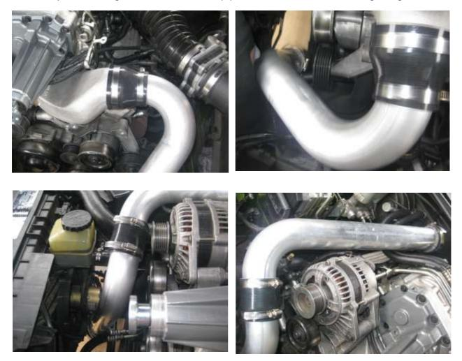
Slight adjustment using cable ties may be required to keep pipe from knocking onto the radiator fan. Also note the location of the hump bellow hose as shown in the image below right.
