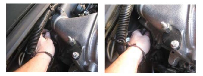
There is a small hose and a larger hose. The larger hose is attached by a clamp which can be removed by hand or using some vice grips.
