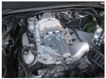
Once supercharger is secure, attach all hoses back onto the supercharger housing and elbow.
