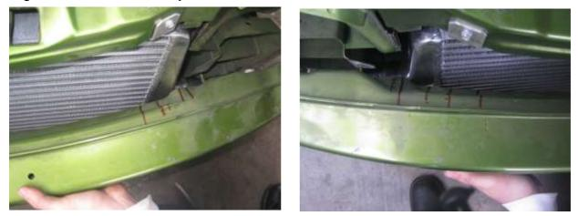
Take notice of the bottom of the reo bar as this may need adjustment too. At the same time roughly position the core outlet piping into place in order to determine where further modification is required.
