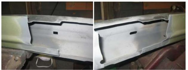
Once the cuts have been made, spray with rust guard and test fit the reo bar onto the car to determine if further cutting is necessary.
