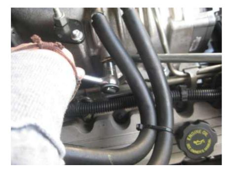
Step 4 – Removing injector cables Using a flat-headed screw driver, unclasp the clips shown below in order to detach the cable from each injector.
