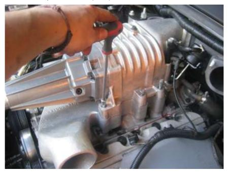
Use a torque wrench to torque the bolts up to 18 Nm
