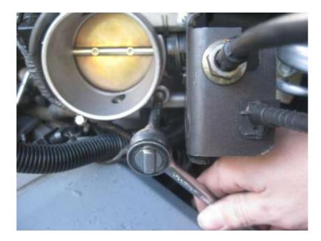
There are 2 bolts which physically hold the throttle body onto the elbow.
