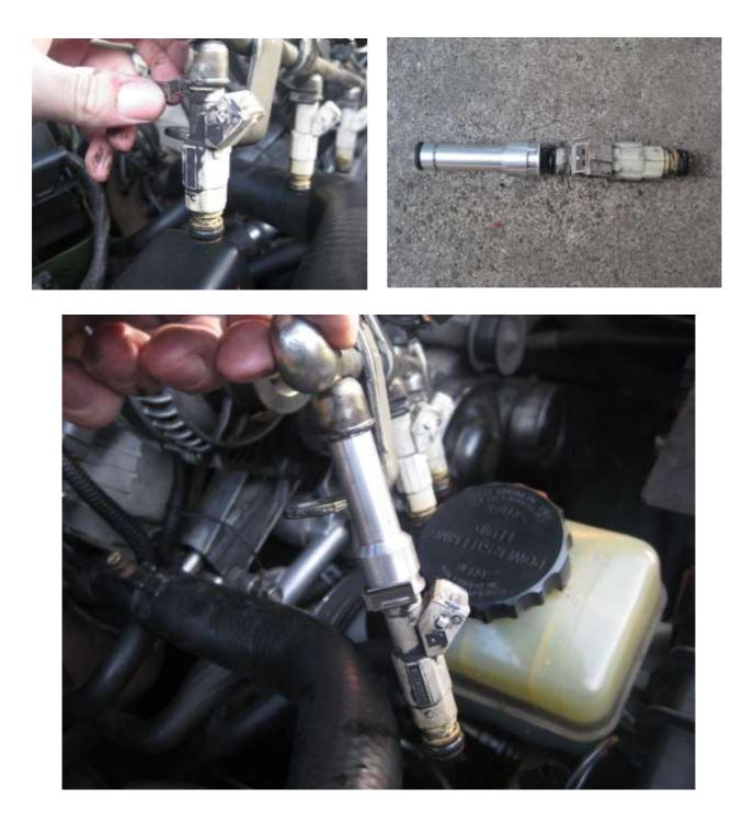
Replace metal clips and use extra clips as provided in order to assemble the injector and extender to the rail as shown below.
