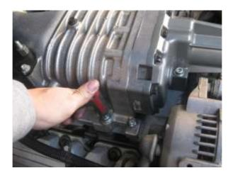
The following three images show the hidden bolts at the back of the supercharger.
