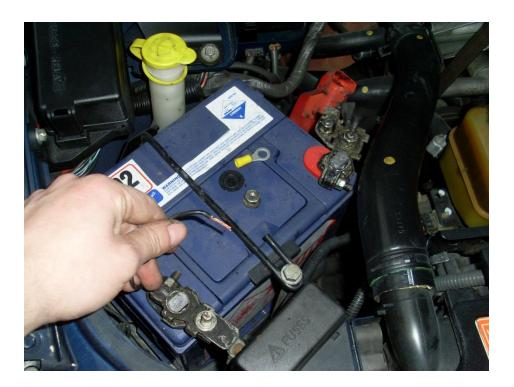
Crimp the eyelet to the wire (using an electrical crimper) and fasten it using the nut on the negative battery as shown below.
