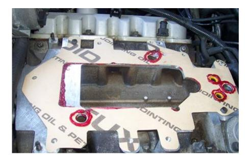
Apply sealant to the bottom of the assembled core (as shown below) and place the assembled core onto the gasket keeping all holes centred using the bolts supplied. Attempt to screw the bolts into place through the core and adjust the core where needed.
