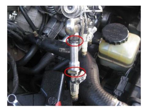
It is important to first connect the injectors into the cylinder heads ensuring all o-rings pop into place. Proceed by carefully wedging the hollow cylinder shafts in between the manifold and the existing fuel rail brackets before placing the 4 bolts through the holes and fastening them.
