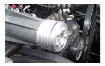
Cut a decent size section out of the sound deadening using scissors and inspect any other areas for interference. Since all cars are different the exact areas and amount of relief needed varies. The bonnet may need to be grinded if it makes contact with the pulley.
