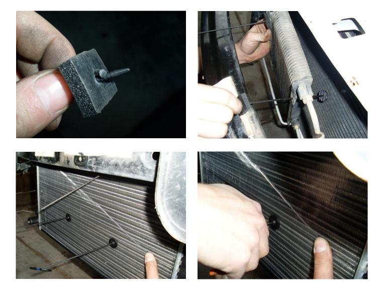
The heat exchanger does not need to be bolted on at this stage and can simply be held up for this fitment. The fins may need to be slightly alleviated (with a thin screwdriver or similar) in order to easily slip the nylon rods through the heat exchanger. Trim the nylon rods back once the locks have been fitted.
