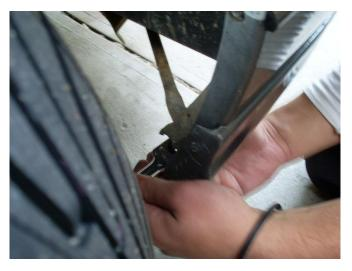
The following images show the screws on the inside of the bumper which need to be removed.
