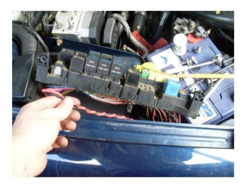
Solder the joined wires and insulate properly using electrical tape
