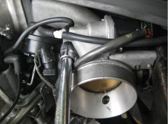
After the throttle body is detached, the bracket must be removed which is now only attached at the throttle and cruise control cable. First remove the cruise control cable by carefully unclipping the plastic clip. Then use a spanner to undo the nut on the throttle cable and slide the cable out as shown below.
