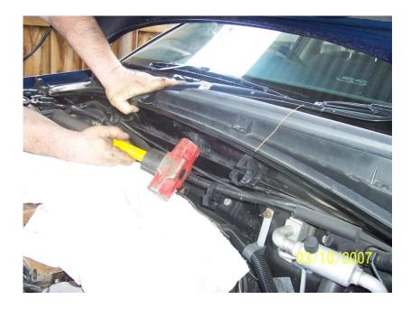
The area shown in red is a point on the firewall which may make contact with the top of the supercharger elbow and may need to be trimmed as required using a jigsaw. Every car is different therefore some cars may need more or less amending.
