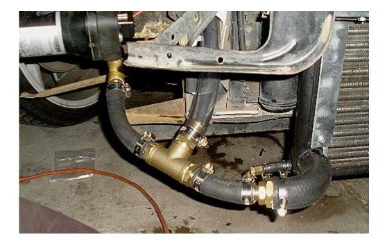
Cut a length of  $\frac{3}{2}$  hose (enough to reach intercooler core) and connect it to the top connection on the pump as shown below.
