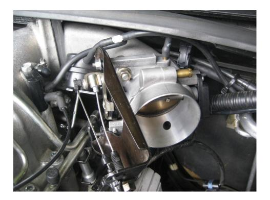
The vacuum hose from the throttle body to the back of the supercharger will no longer reach the supercharger once the throttle body is upside down and will need to be replaced by the supplied longer hose. This longer hose will then need to be spliced and teed (process is shown further down).
