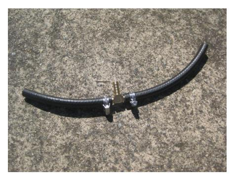
Refit the throttle body (upside down) and fit the end with the shorter hose to the back of the supercharger where the old hose was connected. The nozzle is hard to see but is marked in red below. The other end simply fits into the throttle body as the old hose did.
