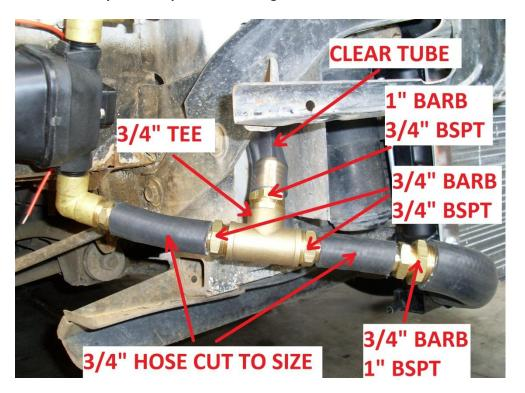
The clear tube is used as a filler tube/water level gauge and should be trimmed at the top to a suitable size. The end should be blocked off using the 1" end plug and secured using a hose clamp.
