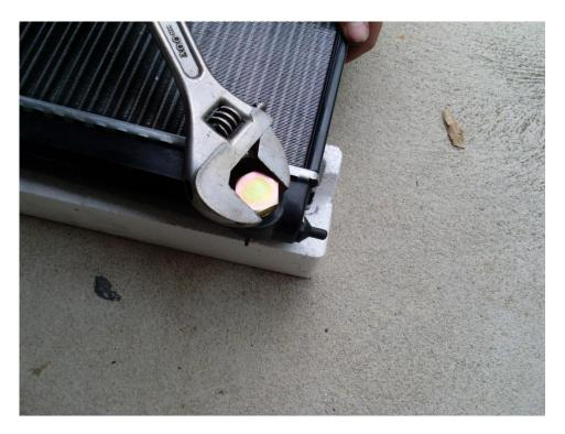
Orientation of the front mount radiator is such that the plug faces outwards on the passenger side of the vehicle.
