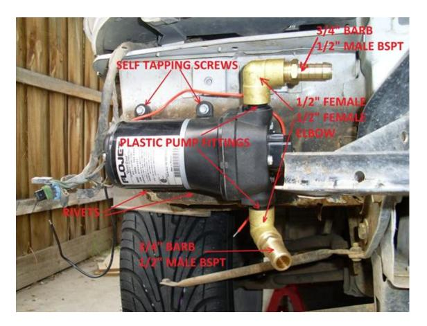
The top side of the pump should be fastened using the provided 5mm self-tapping screws. The bottom side must be secured using rivets, to prevent drilling through the battery behind the bodywork. The rivets are also provided.
