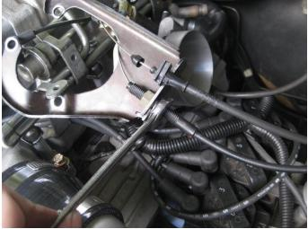
Now remove the clips which connect the cables to the throttle linkage as shown below (a screwdriver may be of help).
