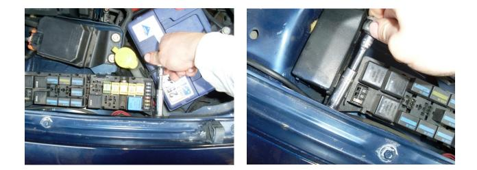
Also release the fuse box by unclipping it using a screwdriver as shown.
