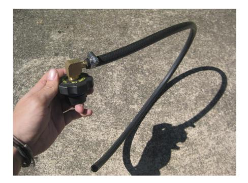
Prepare the connection shown above by using 3/8" Barb ½" Male BSPT Elbow and screwing into the supplied threaded oil cap (using Teflon tape on thread) and secure the 1 metre long hose with a hose clamp as shown below. The other end of the hose will connect to the Tee.
