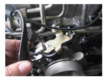
Once the bracket is removed it can be marked (as shown) and trimmed using a hand saw or angle grinder. The bottom arm shown is cut off completely while the top should be grinded down for adequate bonnet clearance.
