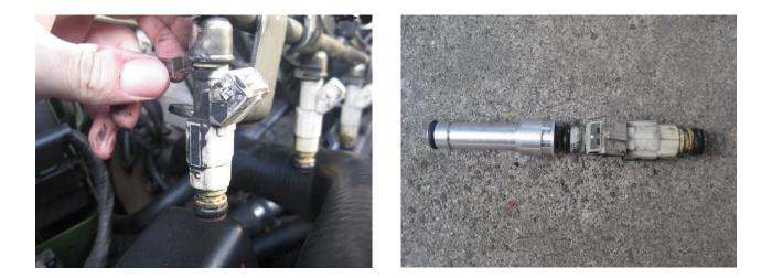
Refit metal clips and use extra clips as provided in order to assemble the injector and extender to the rail as shown below.
