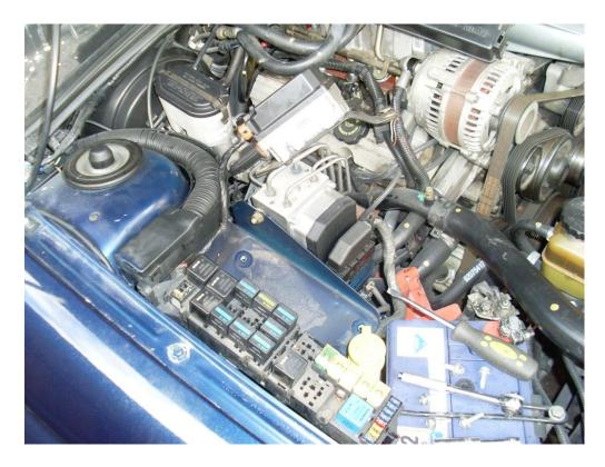
Locate the fuel pump cable and remove some of the rubber lining as shown. NOTE: NOT every vehicle's fuel pump cable is purple; therefore you may need to use a workshop/repair/wiring manual to locate the correct cable or if possible use the fuse diagram on the back of the fuse box cover (where applicable). A relay may also be added.
