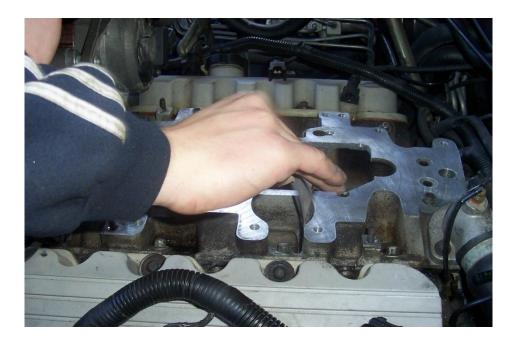
Place the lower half of the intercooler core enclosure onto the inlet manifold making sure all holes are aligned. Mark (using a permanent marker) the hole as shown as it needs to be drilled to 12mm.
