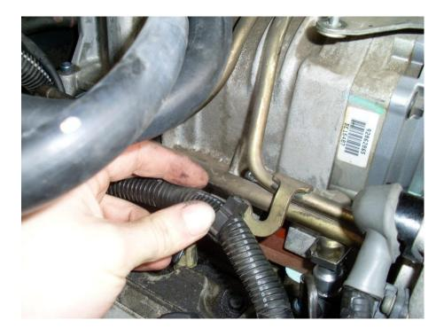
Refit all injector loom clips into the injector rail
