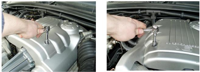
Proceed by removing the injector rails by unfastening all the injector rail bolts. There are 5 areas where the injector rail is fastened as shown below.
