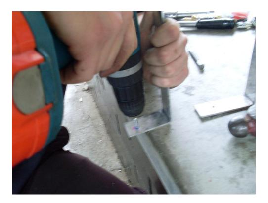
The pre-drilled hole on the bracket is used in conjunction with the pre-tapped radiator mounting holes. The 5mm button headed screws are used to secure the bracket onto the radiator. Repeat this process for both brackets/sides.
