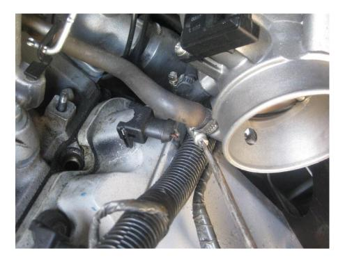
Once all bolts and hoses are removed, the supercharger is then free to be lifted off the car.
