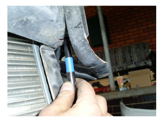
Once the brackets have been marked (shown in blue), begin drilling the holes.
