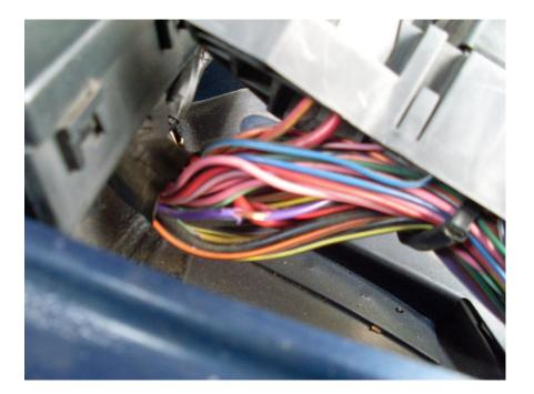
Use the two self-provided electrical wires and join the positive to the fuel pump wire. The other is negative and is simply used as a ground and can be grounded to the battery (shown later).
