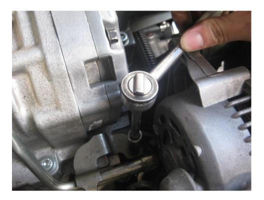
The support bracket for the alternator must then be removed by removing the bolts on the alternator and supercharger.
