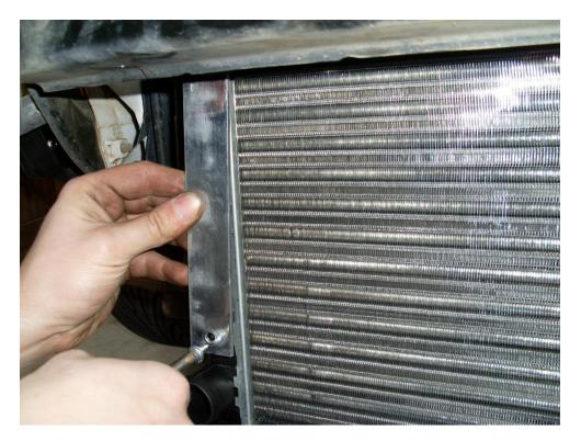
The brackets are mounted to the reo bar using the 5mm self-tapping screws provided. Using a socket wrench, screw them into the reo bar and through the bracket.
