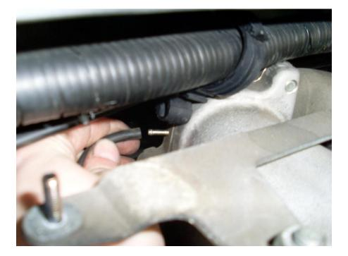
Refit the vacuum brake booster line as shown
