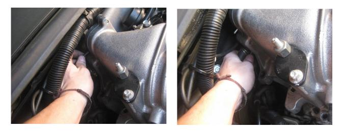
There is a small hose and a larger hose. The larger hose is attached by a clamp which can be removed by hand or using some vice grips.
