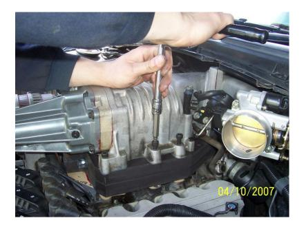
Lightly tighten the bolts using an Allen key or socket wrench to progressively fasten each bolt. Using a TORQUE WRENCH initially torque the bolts to 10Nm before setting the torque wrench to 17Nm and further tightening the bolts. It is CRITICAL not to over tighten the supercharger bolts as the supercharger housing will deform and make contact with the supercharger rotors. Be sure to spin the supercharger pulley by hand to inspect for any rubbing. If rubbing occurs slightly loosen the bolts.
