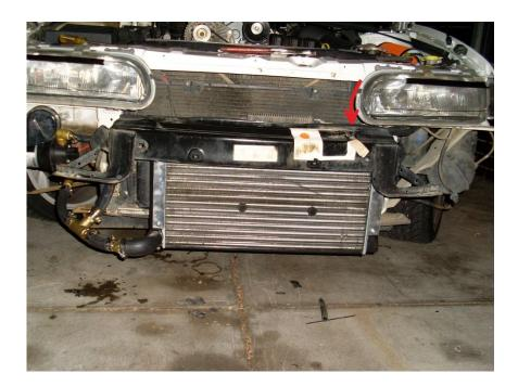
Secure the connection using hose clamps as shown below. Once again cut a length of 3/4'' hose (enough to reach intercooler core) and attach it as shown.
