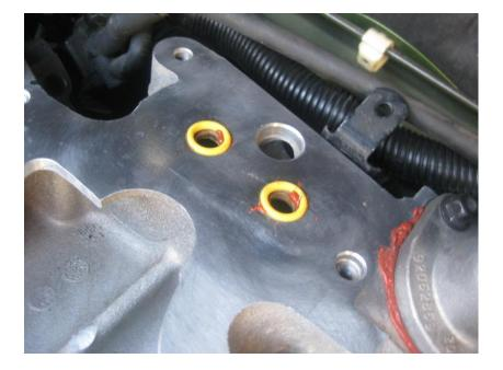
The inlet manifold should ideally be ported as it is causes a restriction when the intercooler core is fitted. This can be done using a jig saw by approximately marking out a path similar to the one shown. Alternatively if you would like the inlet manifold CNC ported, MACE do offer this service which requires that the inlet manifold be removed and posted/dropped to MACE.
