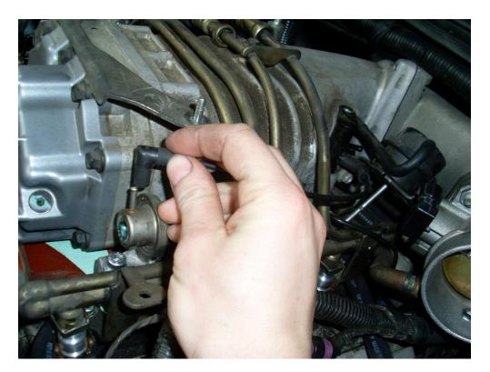
Be sure to BLOCK off the shown nozzle in the vacuum tree using the vacuum block-off plug provided
