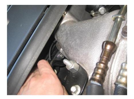
Connect the hose from the oil cap to the tee as shown below. This continues the vacuum process which was previously blocked off by the intercooler core. Secure the Tee fitting using hose clamps as shown.
