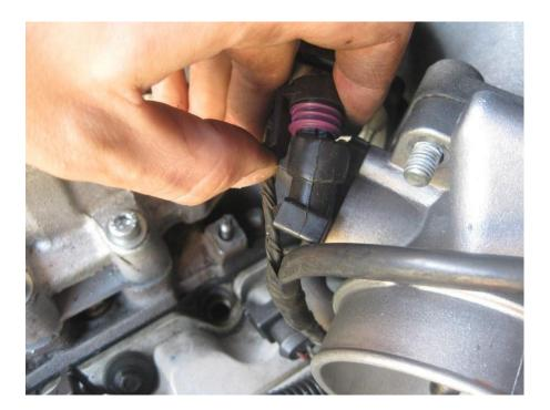
Also remove the plug from the idle air control valve located on the right side of the throttle body.
