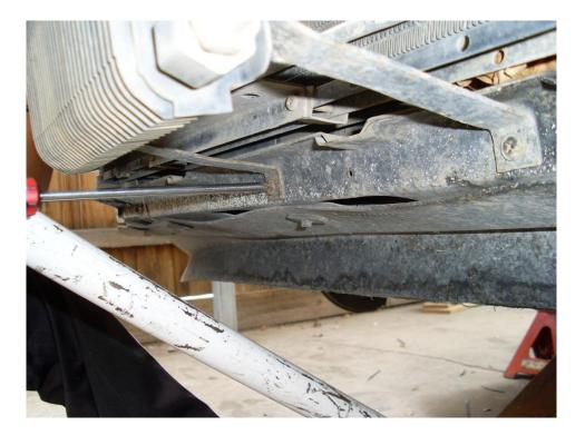
Remove the 2 brackets (top and bottom) behind the transmission cooler by undoing the nuts which retain the brackets as shown below. **NOTE: Keep the oil lines attached as the transmission cooler must not be completely removed in order to be relocated.**
