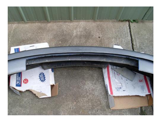
For clearance issues, the bumper may need to be trimmed using a jigsaw or angle grinder. Test fit the bumper bar and using trial and error; locate the areas which need trimming. Refit the bumper and check all connections.
