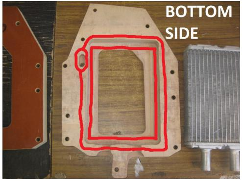
Applying a plentiful amount of sealant is important to prevent air from flowing around the radiator. Apply the sealant to BOTH HALVES of the core as shown below.
