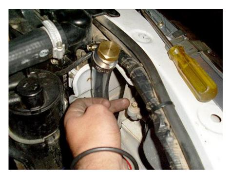
Create a block off for the nozzle on the radiator with the fittings shown below. Block the supplied 5/16" Barb with the 1/8" end plug plug (shown below) again using Teflon tape and secure both using a spanner and a shifter.
