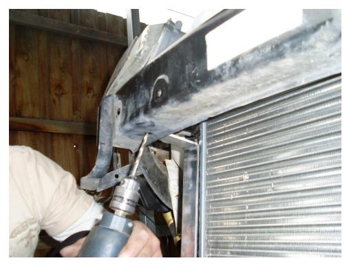
Once the hole is drilled, it is possible to place a mark (using a pencil) on the bracket to locate the position of the hole to be drilled into the bracket.
