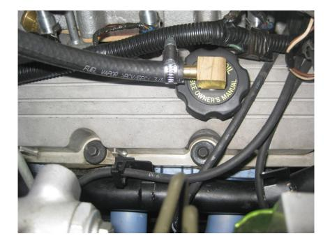
Run the hose behind the back of the engine hiding it as best as possible for a neater look.
