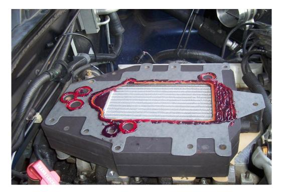
Place the supercharger over the core and locate all inlet manifold holes using the bolts provided. Adjust the supercharger by moving it around until all bolts screw into their respective holes
