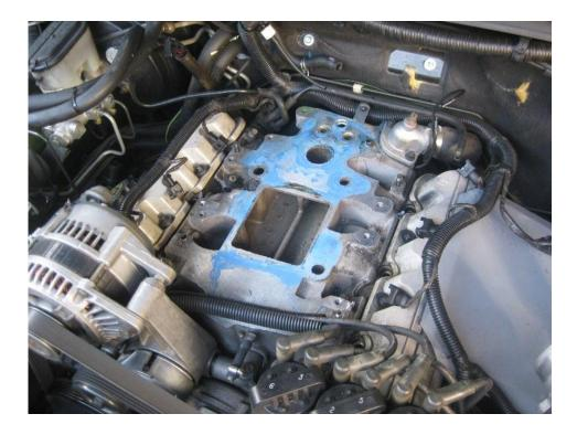
It is a good idea at this stage to tighten the inlet manifold bolts (as shown below) as they can be prone to loosen. These should be torqued up to about 15 Nm.
