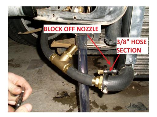
Secure all the fittings using hose clamps as shown below.
