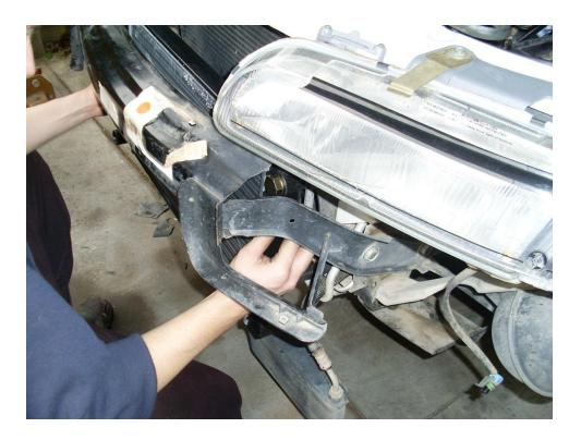
Position the bracket with the LONGER flange onto the driver's side of the radiator and drill a hole into the bottom of the reo bar as shown. The brackets are of different sizes to offset the radiator in order to accommodate for the air-conditioning drier/receiver.
