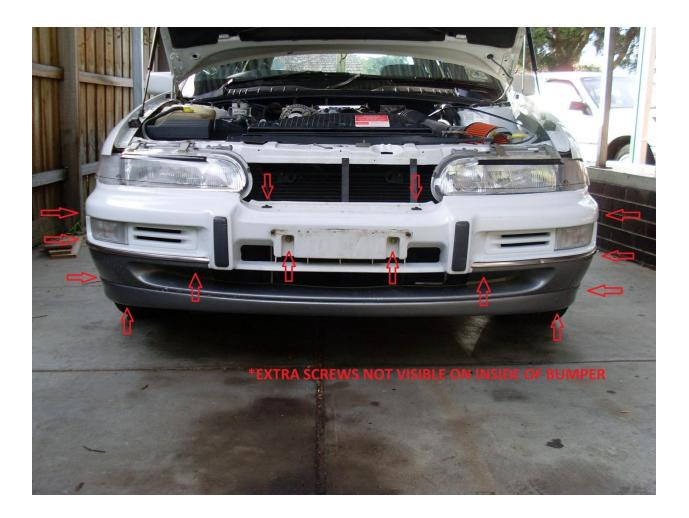
If your vehicle is fitted with 20 inch wheels and/or lowed, it may be helpful to jack up the vehicle and remove the front tyres for easier access to inner bolts.
