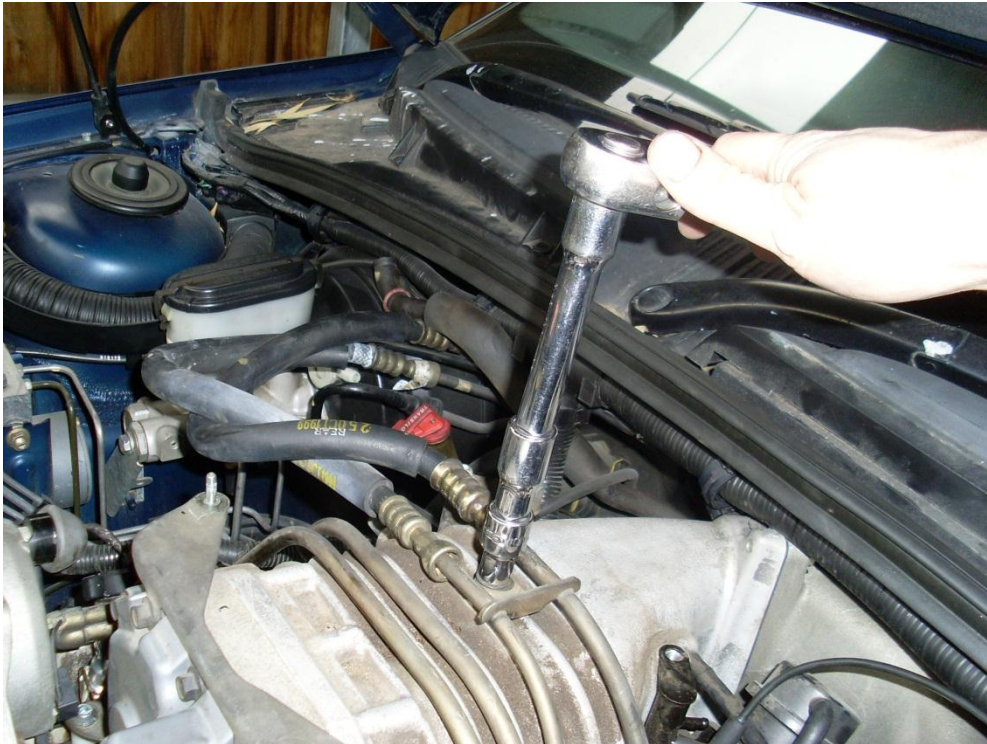
Refit all injector electric clips as shown
