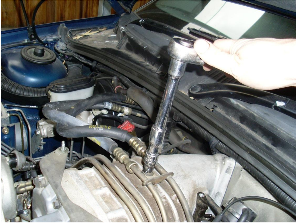
Refit all injector electric clips as shown
