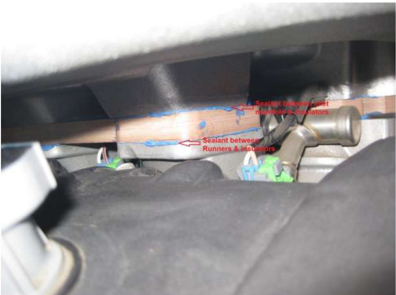
(Picture is to be used as a guide to illustrate how to spread the Silicone over the Manifold Insulator)
