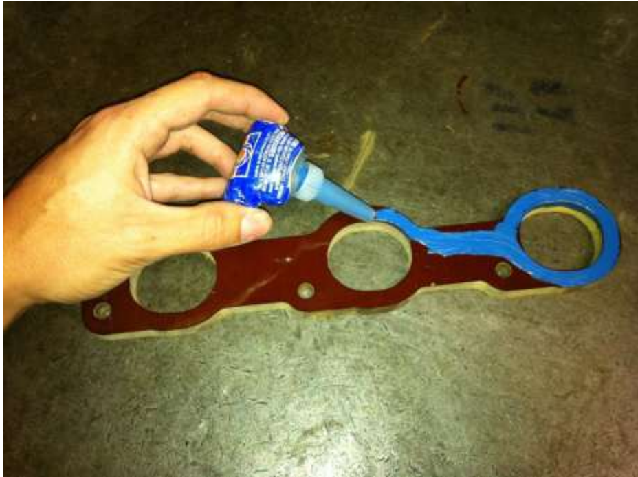
(Picture is to be used as a guide to illustrate how to spread the Silicone over the Manifold Insulator)
