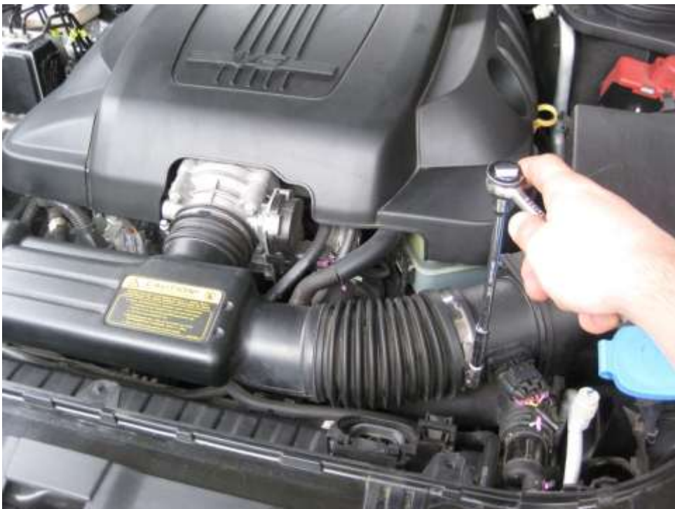
Hose clamp near air box
