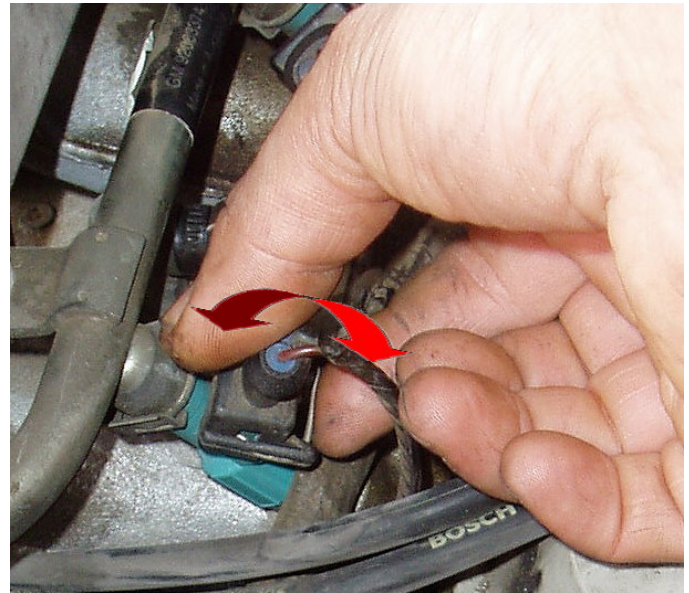
(ii) Rock the clip back and forth until it loosens. Note the injectors are also able to rotate about their own axis, however this will not aid in loosening them.
