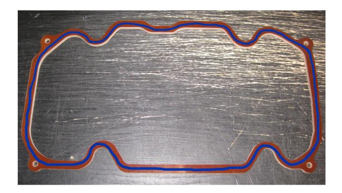
Apply sealant over the factory O-rings onto the manifold bosses and place the supplied spacer bushes over the bolt bosses. Then apply more sealant over the spacer bushes making sure all contacting surfaces are sealed with RTV.
