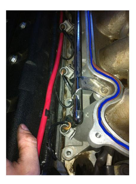
Sealant MUST however be applied to the top face of the Plenum Spacer which mates up to the bottom face of the plenum. Apply the RTV Blue sealant as shown below.
