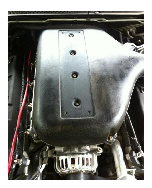
Lastly refit the 'BOSS 260' plate onto the plenum. Allow the sealant a few hours to dry before driving the vehicle.
