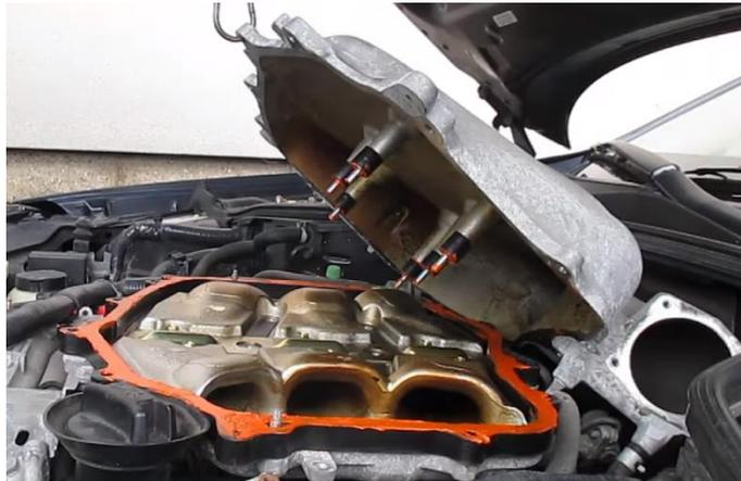
These centre plenum bolts (1 through 6 refer to numbered diagram) will require a drop of thread locker only to the tip of each shortly before threading them in.
