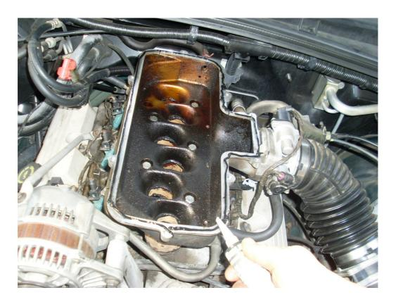
Place the plenum spacer onto the plenum as shown. The plenum spacer is symmetrical across the horizontal axis and will fit the plenum either way.
