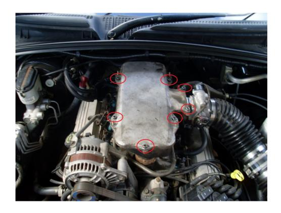
Unfasten the bolts using an Allen key
