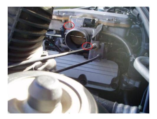
Step 7 - Loosen and remove these nuts.
