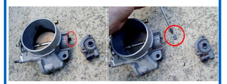
Make sure to save the plastic square sleeve that slides off the shaft end (circled in red).
