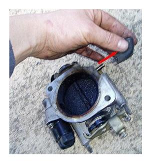
Step 2 - Unscrew and remove the I.A.C valve.
