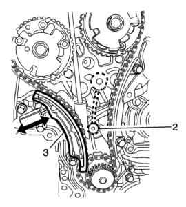
Note: Do not try to force the wedge into position, simply ensure it is loosely engaged in the timing chain and in the correct overall position.
