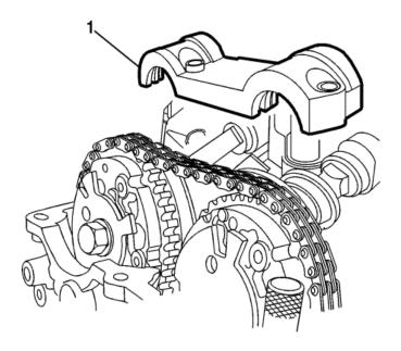
Note: Do NOT remove or loosen any other camshaft bearing caps at this time, even if you intend to eventually remove the camshaft.
