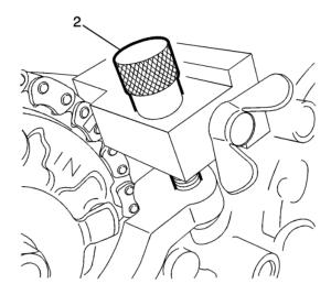
Note: Do NOT over tighten the thumbscrew. The block should be able to slide slightly via the slot the screw goes through. This fore/aft movement will allow easier removal and installation of the chain later.
