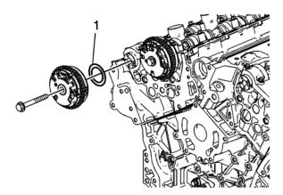
27. Remove and capture the plastic thrust washers (1) in the following steps. Ensure the plastic thrust washer does not fall into the front cover area.
