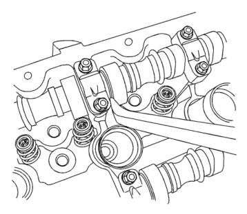
2. It may help to carefully prise the camshaft forward and to move the block backward via the slot to reengage the position actuator to the camshaft. The dowel pin on the camshaft position actuator must be aligned with the slot in the camshaft nose for reassembly.
