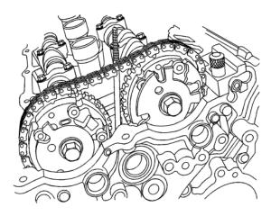
Note: Do not move or disturb the EN49982 retainer components after their installation or the timing chains may be lost inside the front cover.
