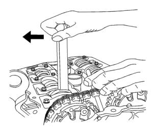
Caution: Be sure the EN49982-2 is captured firmly as described before continuing. This is critical to ensuring the camshaft drive chains stay properly timed.
