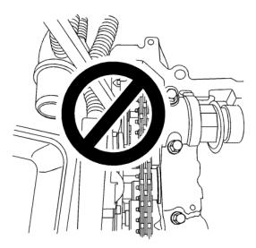
24. Do not prise against the face of the camshaft position actuators or the position actuator retaining bolt.
