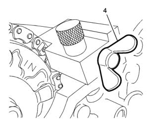
Note: Do NOT tighten the wing nut with a tool of any kind. Firm finger-tightening is sufficient.
