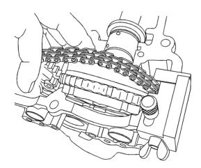
30. Tilt the camshaft position actuator forward and out/away from the engine.
