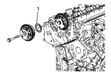
1. Install the plastic camshaft position actuator thrust washer (1) between cylinder head face and camshaft position actuator on assembly.
