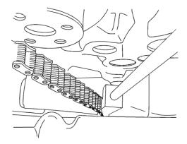
19. If possible, shine a strong light down from above, between the camshaft position actuators, and see the wedge in overall position as shown in the above graphic.
