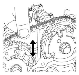
23. With the wedge in position and with the 20 mm wrench removed, there should now be some slack in the timing drive chain as indicated in the graphics shown.
