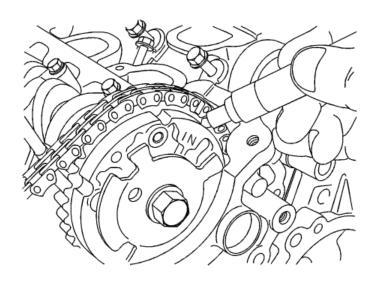
Note: Be certain to clearly mark the position of the chain to the camshaft position actuator(s). Though the engine does not need to be set to a specific timing mark before starting the procedure, the relationship of the chain to the actuator(s) is critical and must be re-established on assembly.
