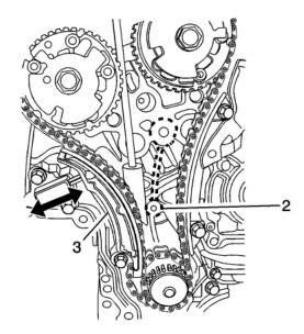
21. This rotation of the camshaft will compress the tensioner shoe (3) against the spring force of the tensioner, opening up a gap between the chain and the internal rib in the front cover. The wedge will then drop into this gap. You will feel a distinct click as the teeth engage the chain.
