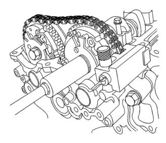
28. To remove the intake camshaft position actuator, remove the loosened retaining bolt. To remove only the exhaust camshaft position actuator, skip the steps for removing the intake camshaft position actuator. However, the block MUST be installed as discussed even if the intake side will not be serviced or the timing of the camshaft chains will be lost.
