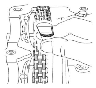
17. Once the rippled portion of the wedge is below the camshaft position actuators, rotate the wedge until the flat in the handle faces toward the intake camshaft position actuator. This orients the "teeth" toward the chain.
