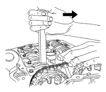
20. Using a 20 mm wrench on the cast hexagonal portion of the exhaust camshaft, rotate the camshaft toward the intake camshaft while pushing down on the handle of the wedge.
