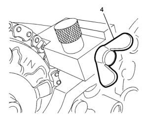
12. Loosen wing nut (4) to open the clamping area of EN49982-1 retainer.
