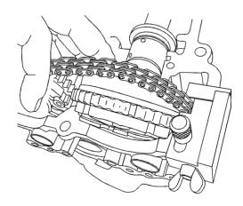
Note: Ensure the plastic thrust washer is in place before installing the actuator.
