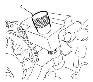
12. Unscrew the wing nut on the block to release the timing chain, and then remove it from the front cover by unscrewing the thumbscrew (2).
