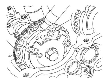
9. Mark the position of the chain to the camshaft position actuator - exhaust.
