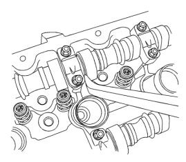
Caution: Do not prise against the face of the camshaft position actuators or the position actuator retaining bolts as the position actuators will be damaged.
