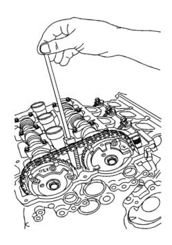
16. Insert the wedge between the two camshaft position actuators with the "teeth" on the wedge facing toward the front cover.
