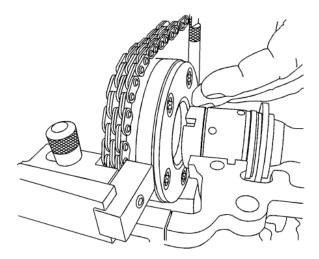
29. Slide the camshaft position actuator forward and off the end of the intake camshaft. The slot in the block will allow the tool to move forward enough to disengage the camshaft position actuator from the front of the camshaft. Remove the plastic thrust washer when removing the camshaft position actuator from the end of the camshaft.
